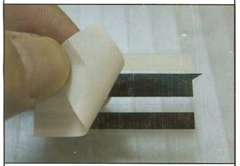
2. Set one of the two separated tapes on a positioning guide, and stick the cover tape downward. (A row of feeding holes must be along a positioning guide.)
