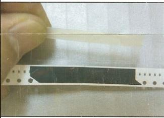
6. Finally, rub joint area of the Joint Tape in a finger. All Completed.
