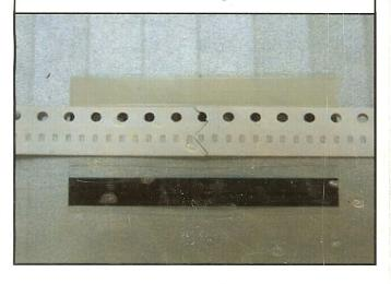
4. Bend the Joint Tape along a bending line and stick it on the back side of carrier tape.
