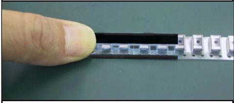
9 Peel a transparent tape from L side to R side of the Joint Tape.
