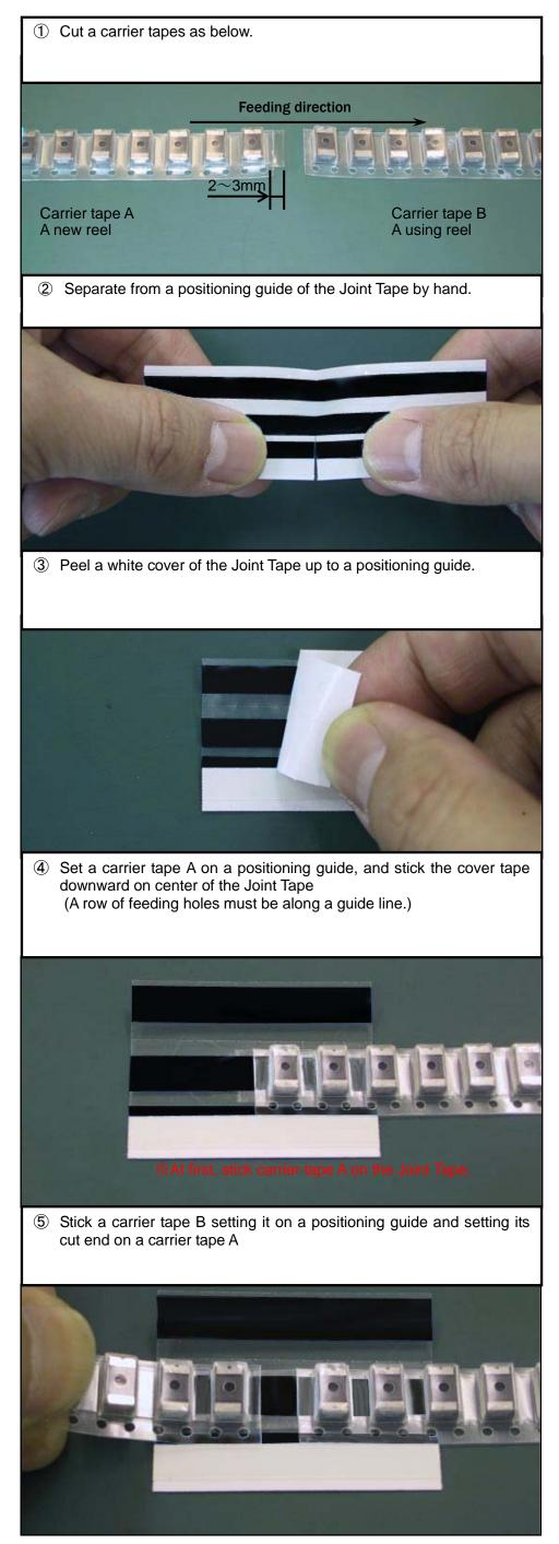
6 Bend the Joint Tape along a bending line and stick it on backside of a carrier tape.
