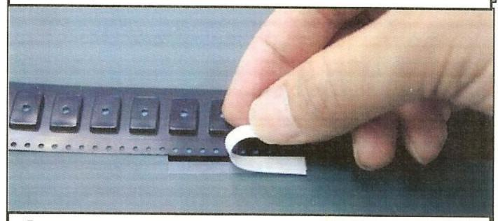
⑧ Bend the Joint Tape along a bending line and stick it on feeding holes side
