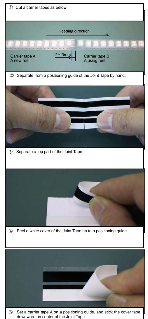
(A row of feeding holes must be along a guide line.)
