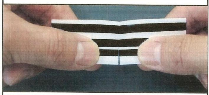
③ Peel a white cover of the Joint Tape up to a positioning guide.
