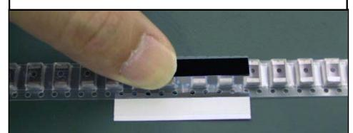
O Peel a white cover and a positioning guide of the Joint Tape
