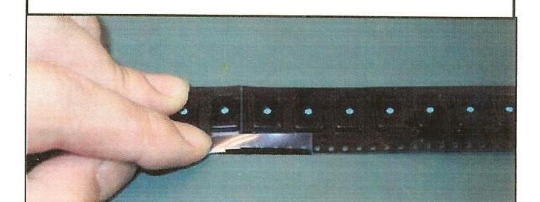
④ Set a carrier tape A on a positioning guide, and stick the cover tape downward on center of the Joint Tape (A row of feeding holes must be along a guide line.)
