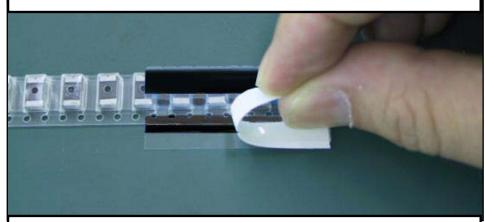
(8) Bend the Joint Tape along a bending line and stick it on feeding holes side
